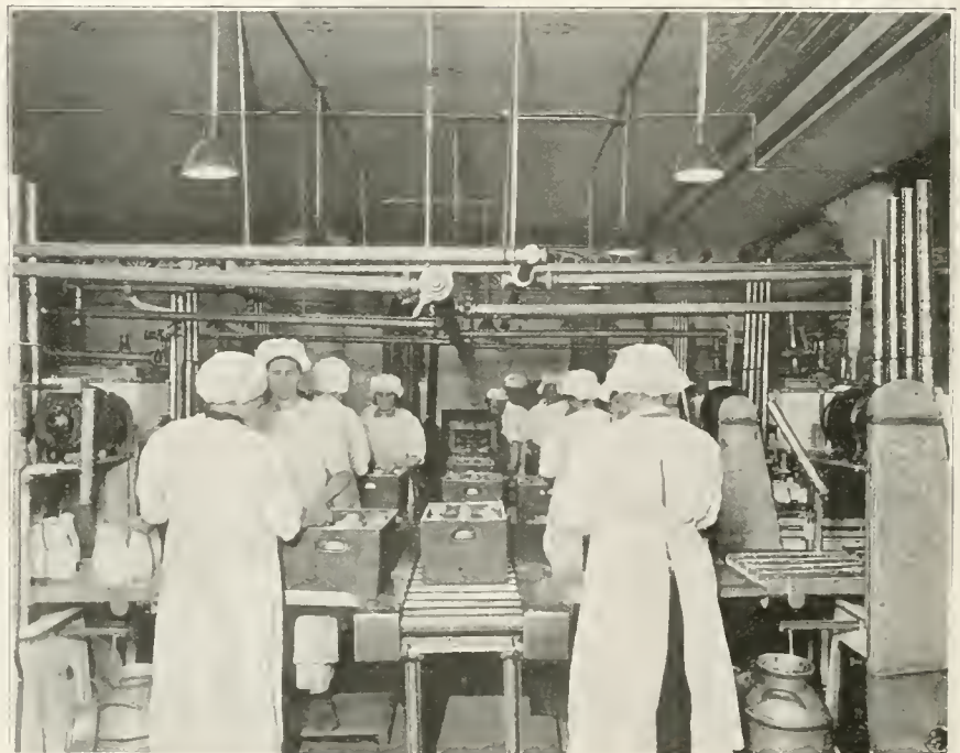
Bottling room, where twenty thousand bottles per hour are automatically filled and capped. Along the route by which the bottles are carried on a moving belt each bottle is flushed with thirty gallons of hot water under thirty pounds pressure.
